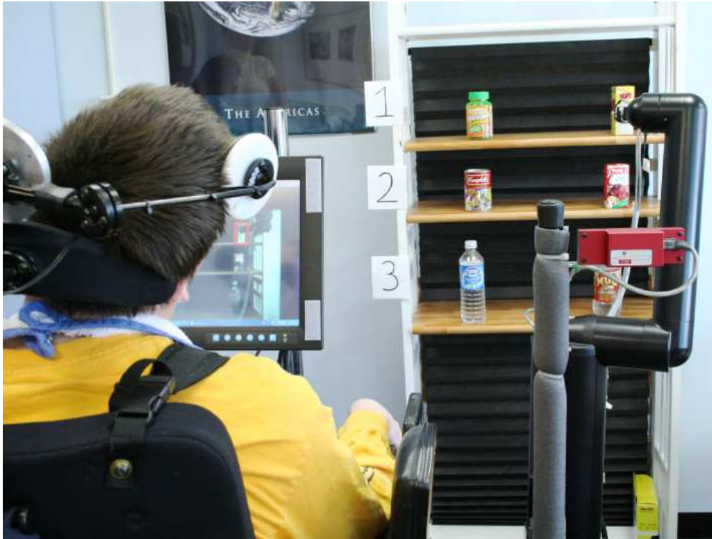
Figure 9.: Experimental setup with single switch scanning. P5 used Cross Scanner (35) single switch scanning software and activated the scanning with a head switch.
