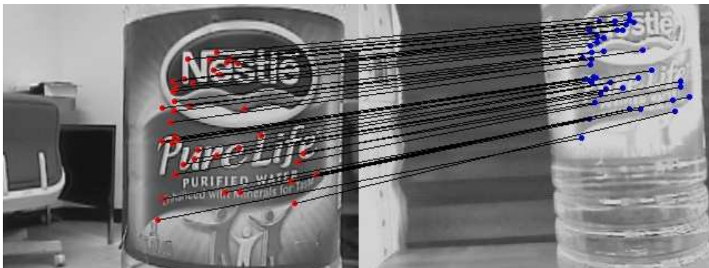
Figure 7.: Object recognition: a successful match between template (left) to current gripper camera view (right) after gross motion and visual alignment.
