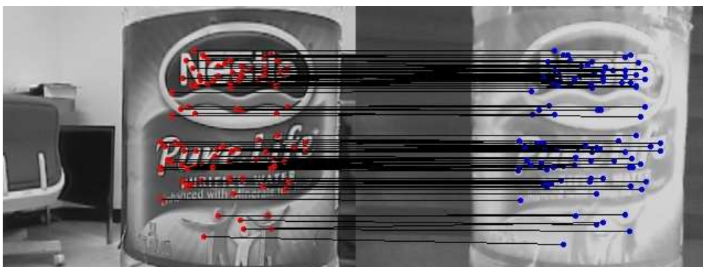
Figure 8.: Successful fine motion alignment between template (left) and left gripper camera view (right). (Best viewed in color.)
